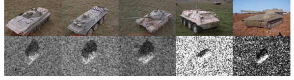
Figure 1. Sample images for 5 out of 10 classes in the MSTAR data set. First row shows the illustrative real life images and second row shows the SAR images from the data set.
